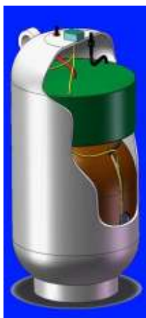
Totally sealed battery module with a ZnCl electrolyte and zinc and tungsten electrodes
